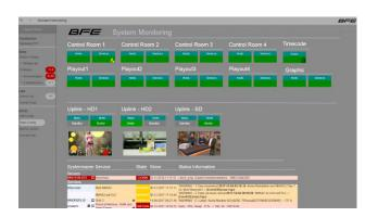
KSC SinAlarm is able to centrally map and monitor, not only standard IT system environments, but all broadcast / media technology environment resources (e.g. routers, video servers, mixers, audiovisual components, servers). KSC SinAlarm helps administrators to detect system problems before a failure occurs. It also eliminates these problems and thus increases the availability of the entire system and the satisfaction levels of users alike.
